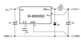
C<sub>1</sub>:  $50V/1000\mu$ F C<sub>2</sub>:  $50V/1000\mu$ F C<sub>3</sub>:  $0.01\mu$ F
